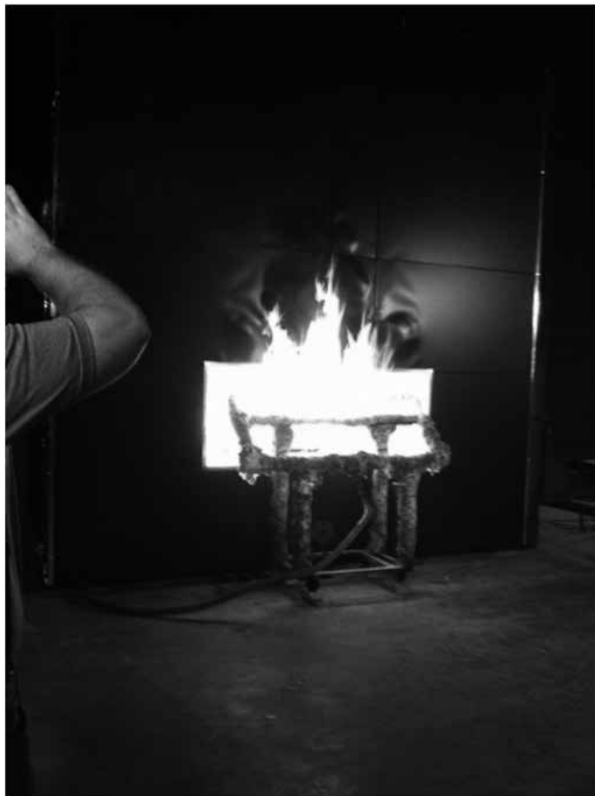
NFPA 285 test determining the fire propagation characteristics of exterior wall assemblies and panels
